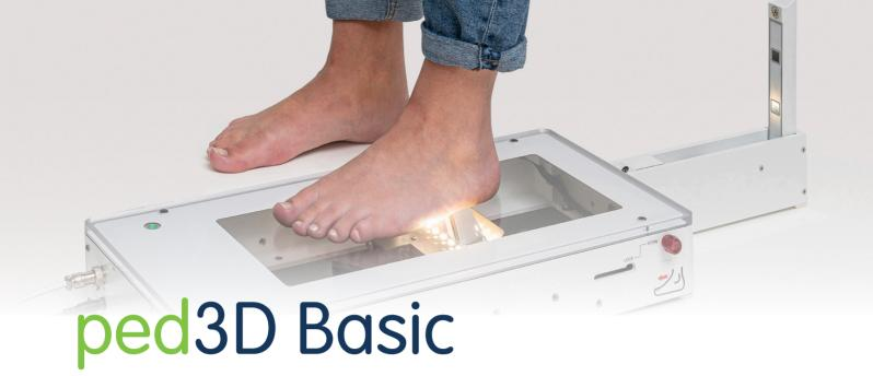
The ped3D Basic Scanner measures the shape of the sole of the foot and provides the obtained 3D data in digital form. This 3D scanner is particularly helpful for the production of insoles for diabetics and rheumatics. Both foot foams, insoles and feet can be digitised with
